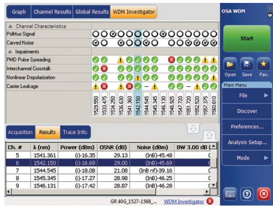
Figure 104. WDM Investigator reading showing a non-linear depolarization contributing to extended noise (OSNR e ).
