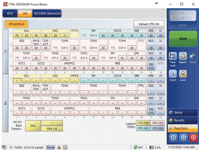
Figure 35. OTN overhead configuration.
