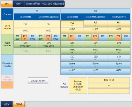
Figure 43. GFP-T overhead-byte analysis interface on EXFO's FTBx-88200NGE OTN analyzer.
