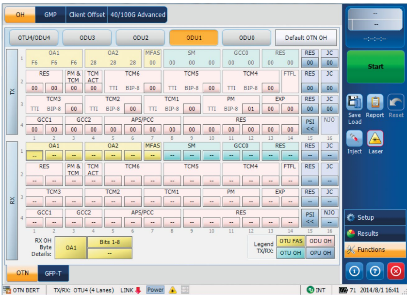
Figure 46. ODUflex overhead byte analysis interface on EXFO's OTN analyzer.
